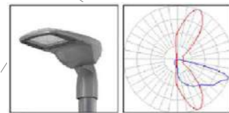
REF A: Kirium Pro Mini, Direct Post, 4 x 350mA 2.7K CLO LED Array, A2 Optic, RAL7046 Grey Finish, 35lux Photocell. 4m TLS Tubular Steel Column, RAL7046 Grey Finish
