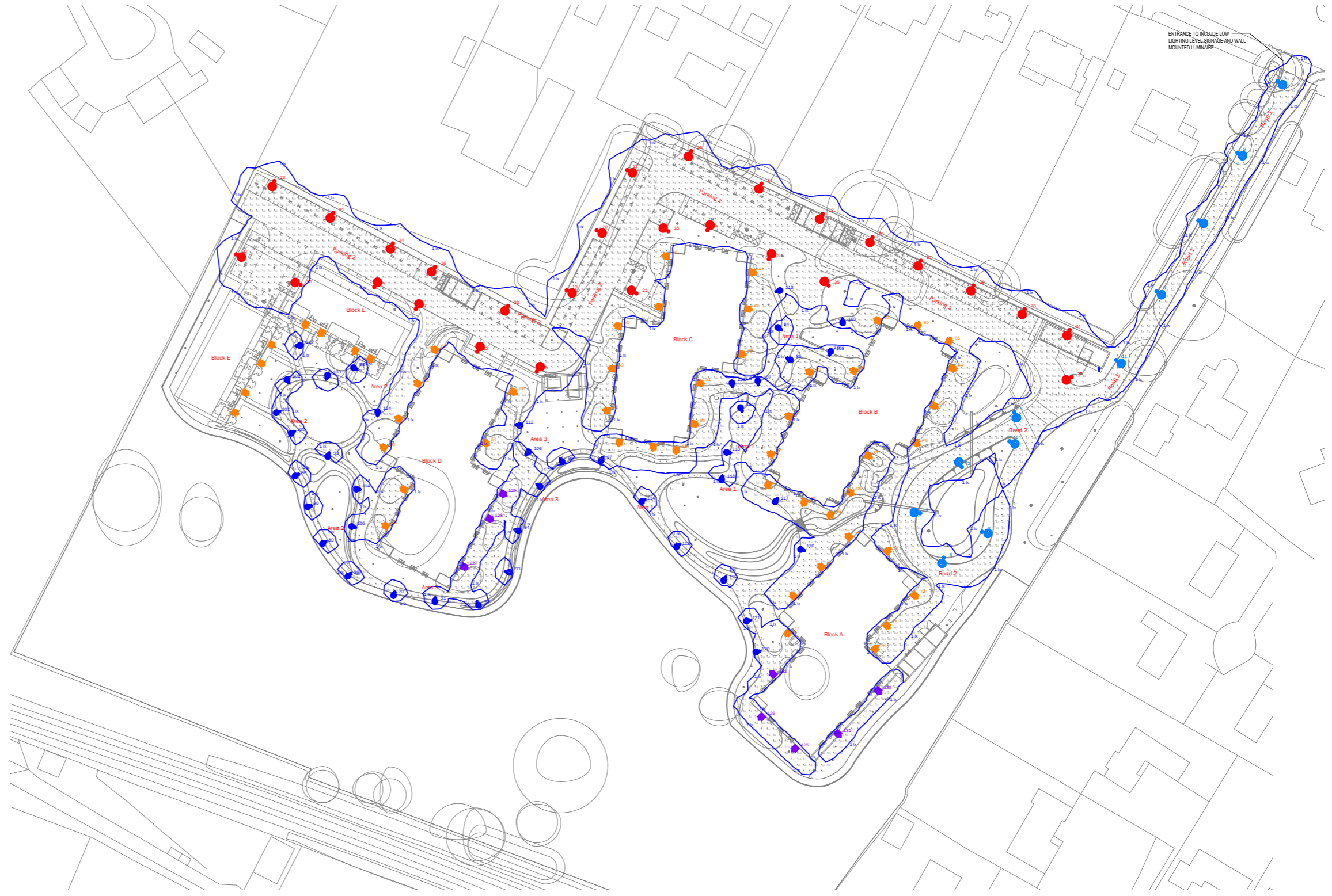
REF A: Kirium Pro Mini, Direct Post, 4 x 350mA 2.7K CLO LED Array, A2 Optic, RAL7046 Grey Finish, 35lux Photocell. 4m TLS Tubular Steel Column, RAL7046 Grey Finish
